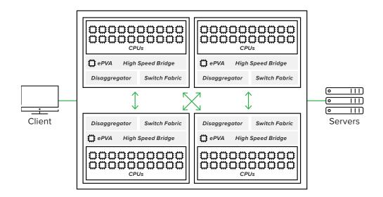
VIPRION 2400 and VIPRION 2200 chassis: The VIPRION 2400 chassis can support up to four 2150 or 2250 blades. The VIPRION 2200 chassis can support two 2150 or 2250 blades. The VIPRION 2250 blade has 10 processor cores (a total of 20 hyperthreaded logical processing cores), and the VIPRION 2150 blade has four processor cores (a total of eight hyperthreaded logical processing cores).
